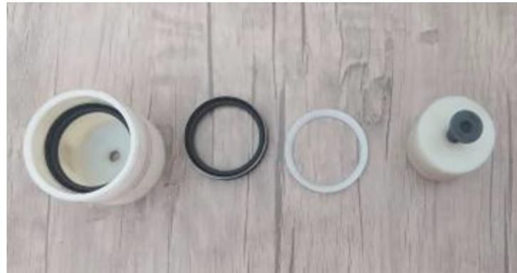
**Figure 1.** Different components of the plunge-cylinder suspension system
